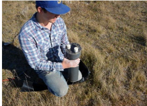
Installing a magnetometer during an MT survey.
