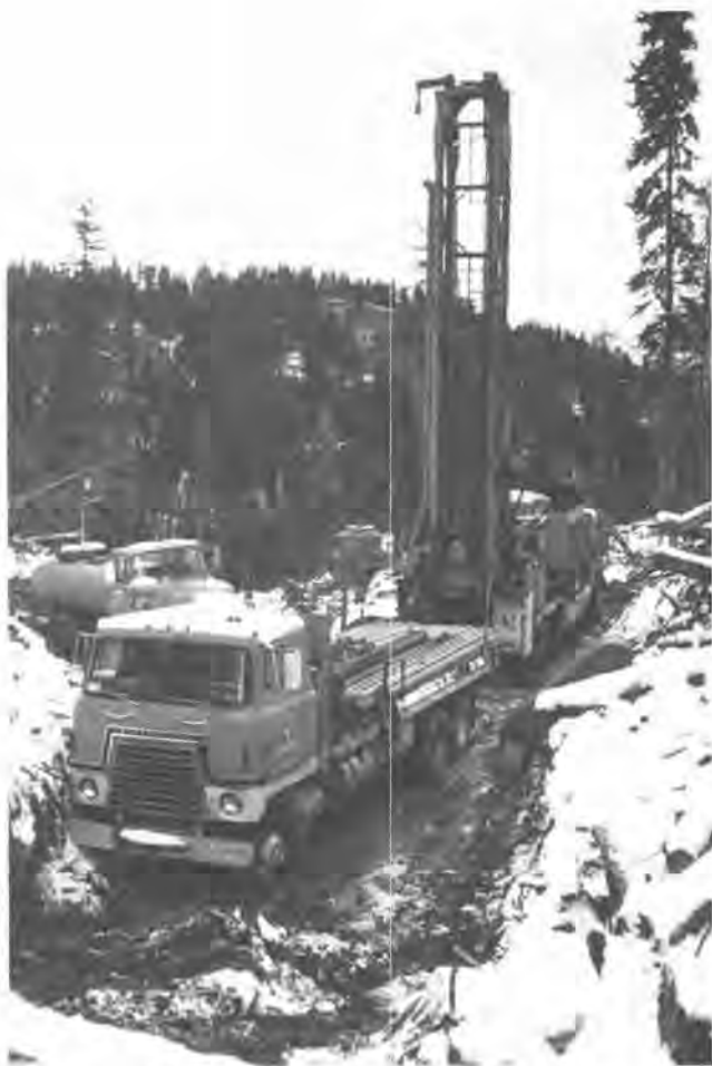
Figure 6. Reverse circulation drill at the Buckhorn Mountain project. Crown Resources Corp. drilled more than 150 rotary holes at the property in 1989. (Photograph by Raymond Lasmanis)
