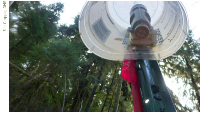
Photo 1. Temperature and humidity logger
