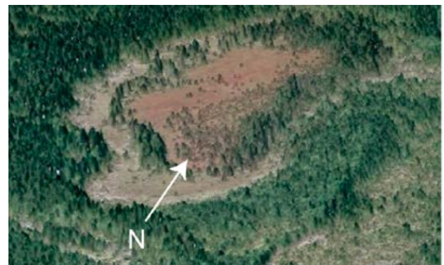
Figure 3. Oblique view of an aerial image that was draped over a LiDAR-derived, digital terrain model of Crowberry Bog. Note the abrupt change in tree height where the plateau begins. The plateau surface is approximately 450 meters long in the north-to-south direction.
