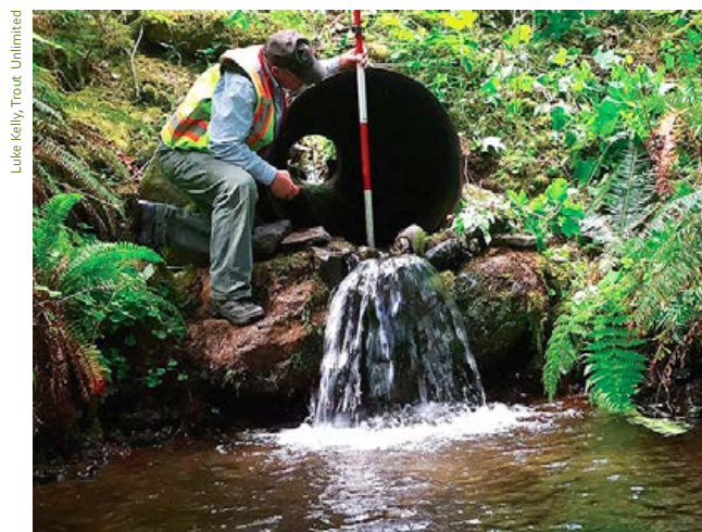
Figure 1. Culvert evaluation. A surveyor measures the dimensions of a culvert pipe to determine fish passage status at this location on the western Olympic Peninsula.
