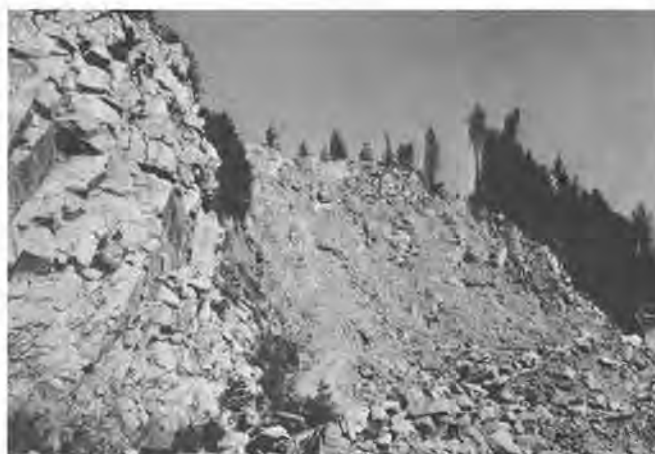
FIGURE 72.—Working face of the Skykomish quarry, in King County, Washington. Quarry is in granodiorite. Quarry is worked only periodically, and broken rock is stockpiled on quarry floor.
