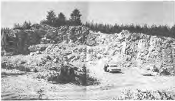
FIGURE 66.—Denny-Renton silica quarry, in King County, Washington. Purest rock is in center of quarry. Dark color of rock at right and left edges of quarry is caused by oxidation of iron.
