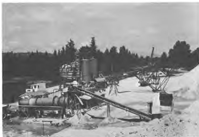
FIGURE 65.—Smith Bros. Silica Sand Co., Inc. processing plant at Ravensdale, King County, Washington. Plant scrubs and dries sand.
