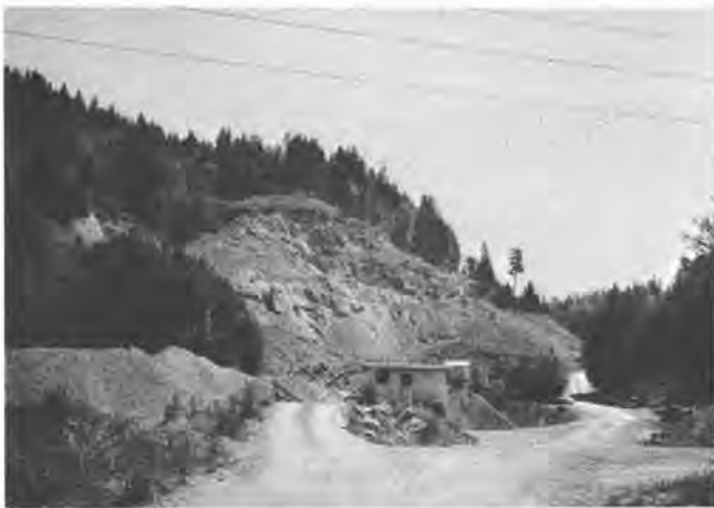
FIGURE 73.—Sunset quarry, near Issaquah, King County, Washington. Quarry is being worked on several levels in an andesite breccia.
