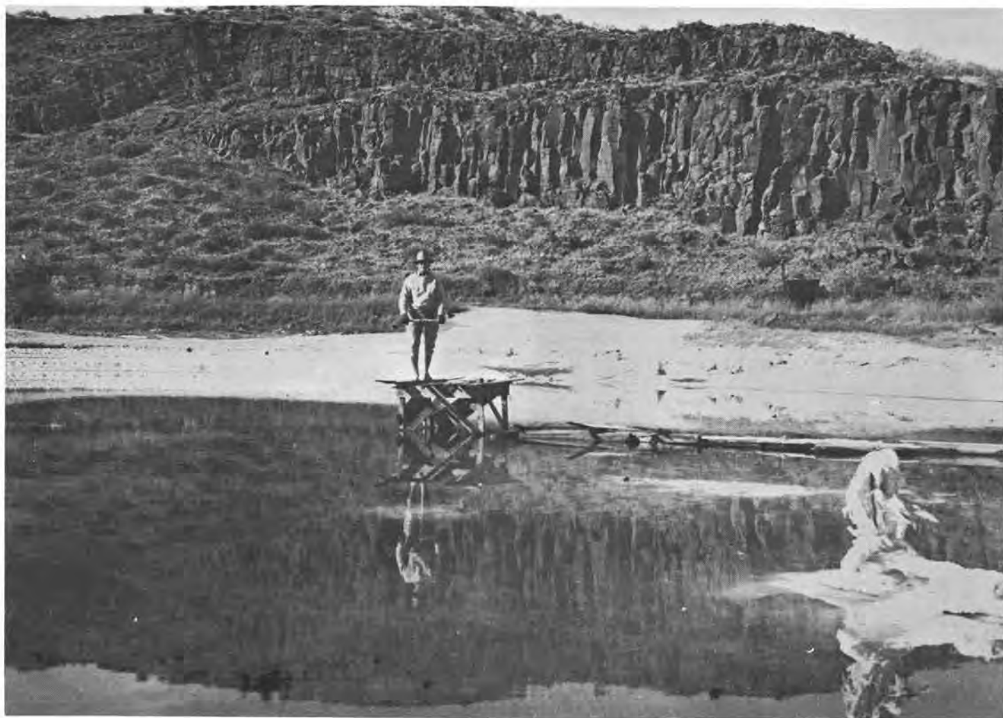
Figure 8.—West side of main brine pool at Carbonate Lake. Note disintegrated wooden post encrusted with salts in right foreground, columnar basalt in background, and hole 12 being drilled from platform.
