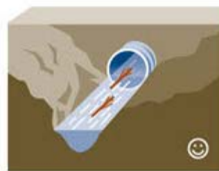
Figure 17 Design to prevent culvert plugging hazard
