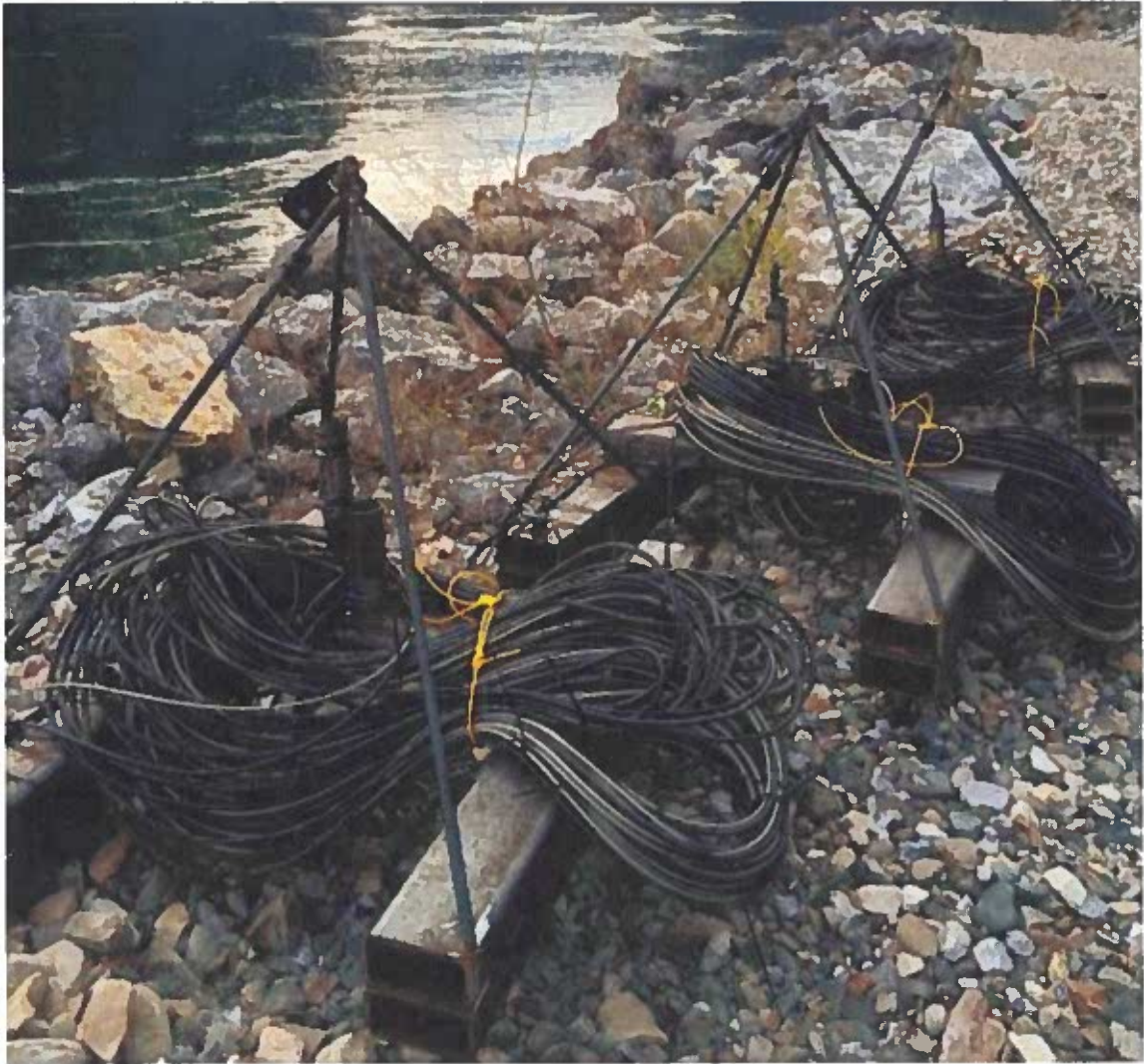
Figure 3. Photo of the heavy mounts (with hydrophone and cable attached) used for tailrace hydrophone placement for the Boundary Project telemetry monitoring.
