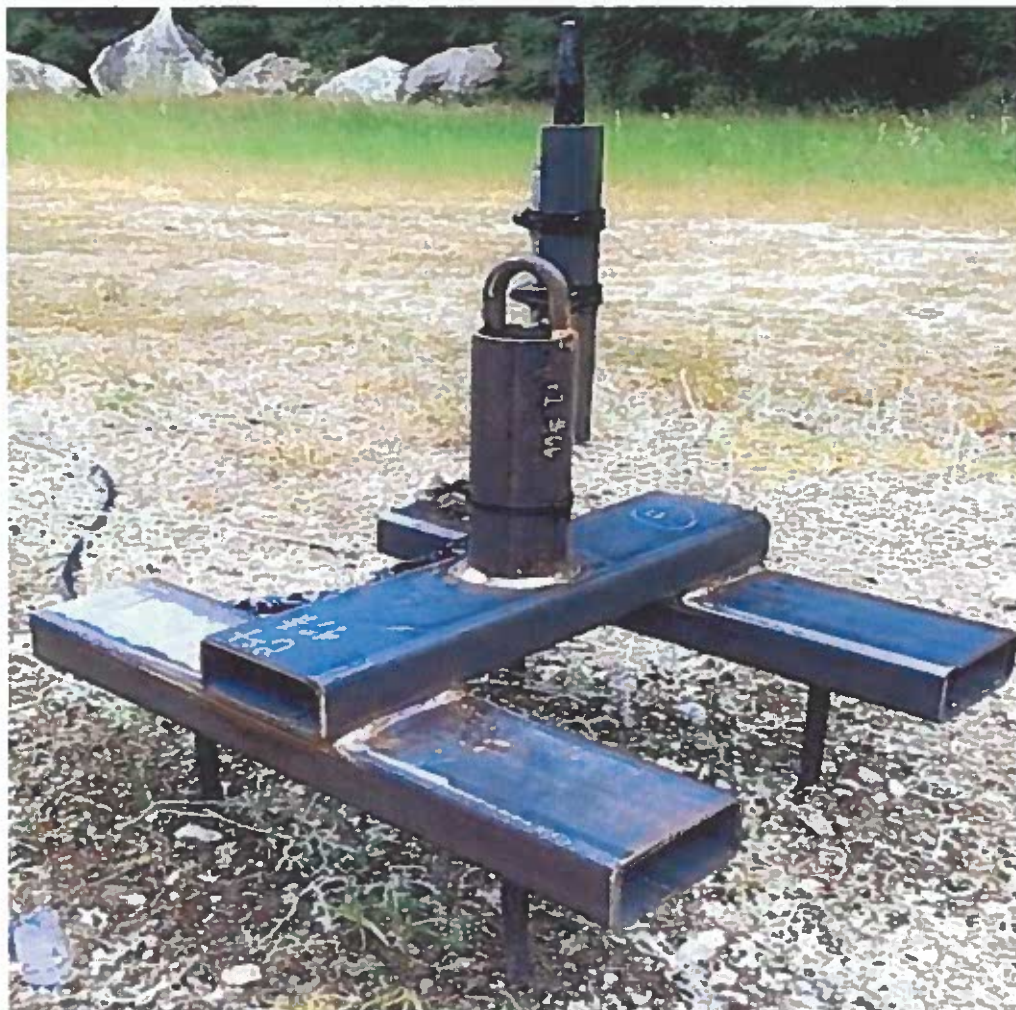
Figure 4. Photo of the mount (with hydrophone and cable attached) used for monitoring sites in the Boundary Dam forebay and tailrace reaches for the Boundary Project telemetry monitoring project.
