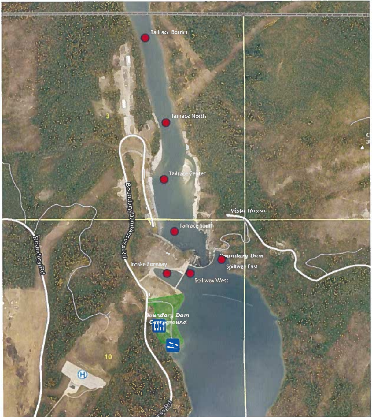
Figure 2. Locations of the seven acoustic tag detection hydrophone mounts places in the tailrace and forebay of Boundary Dam.
