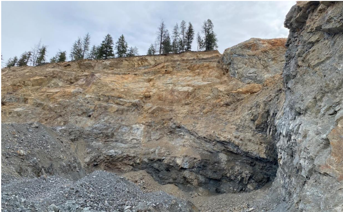
VIEW EAST INTO THE "BOX CUT" OF CUT 1. NOTE THE DARKER, FINE-GRAINED STRATA (THIN SANDSTONE BEDS AND SLATE) AT THE BOTTOM OF THE CUT.
