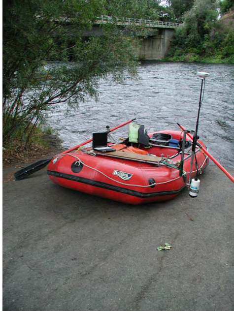
Figure 2B. Picture showing ADP and GPS mounted on the side of a raft.
