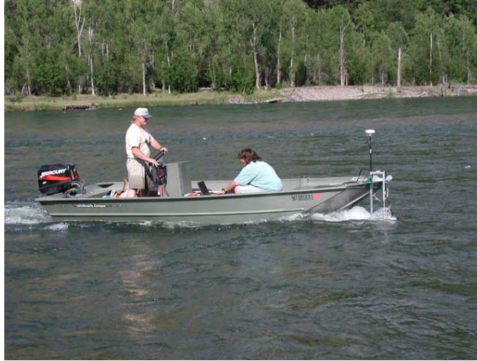
Figure 2A. Picture showing ADP and GPS mounted on the front of a Jet Boat.
