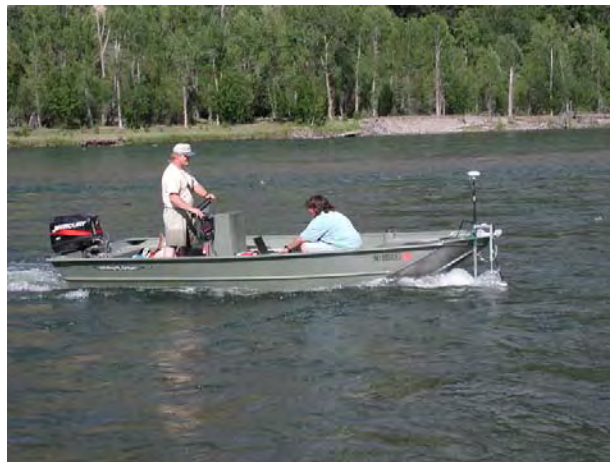
Figure 2A. Picture showing ADP and GPS mounted on the front of a Jet Boat.
