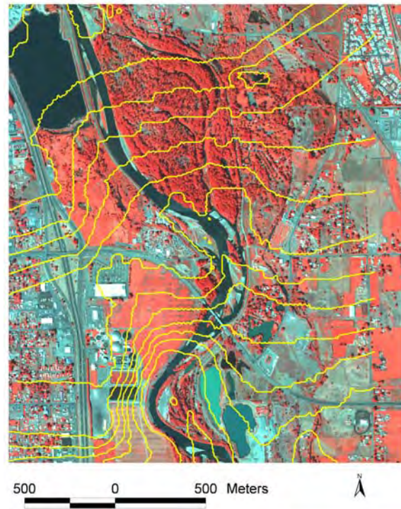
Figure 4. 1 meter contour intervals derived from the 30 m 2 DEM data available from the U.S.G.S overlain on the multispectral imagery from the Union Gap reach. The contour intervals that overlay the water surface allow a first order estimate of river slope.
