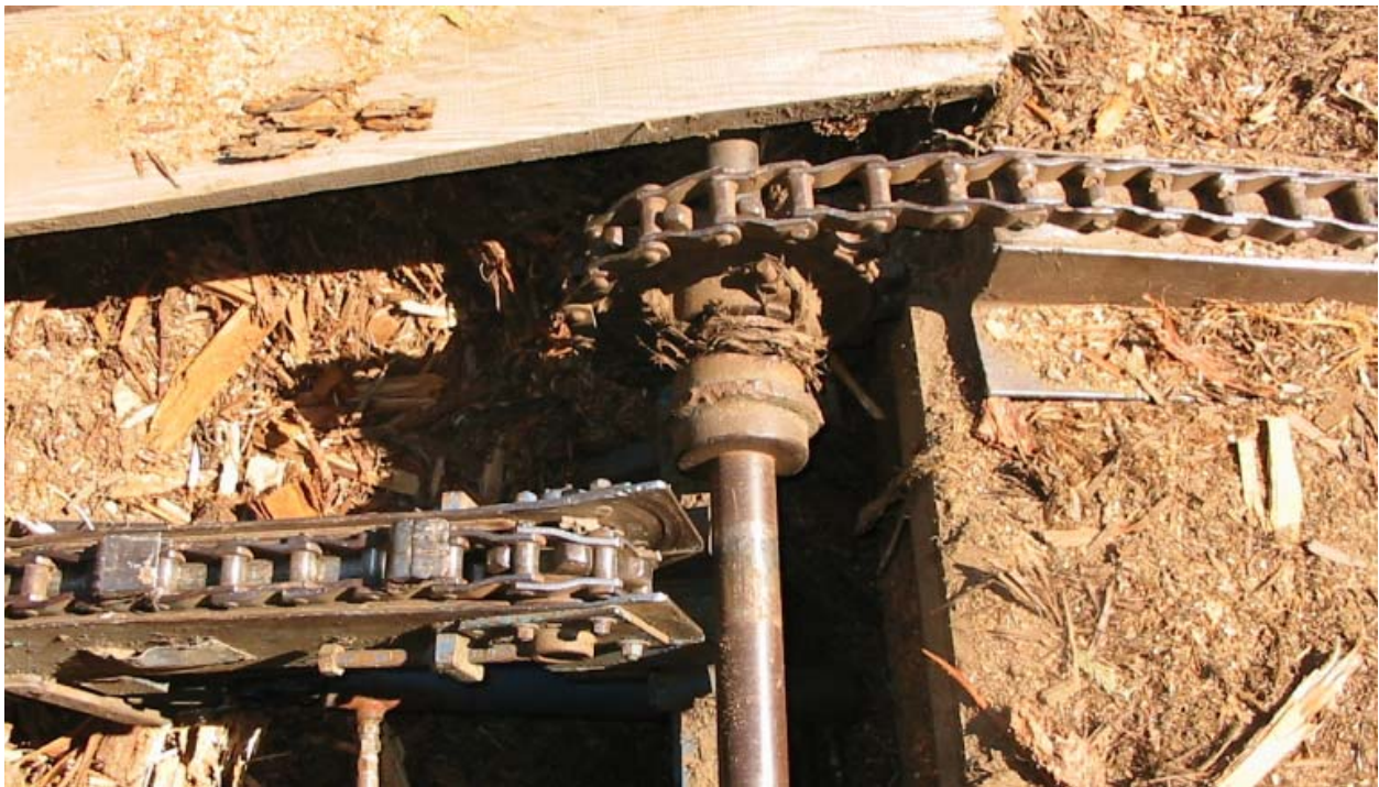
This chain-driven conveyor (surrounded by mill residue) from Monty Pfaff's mill moved logs to and from the saw.
