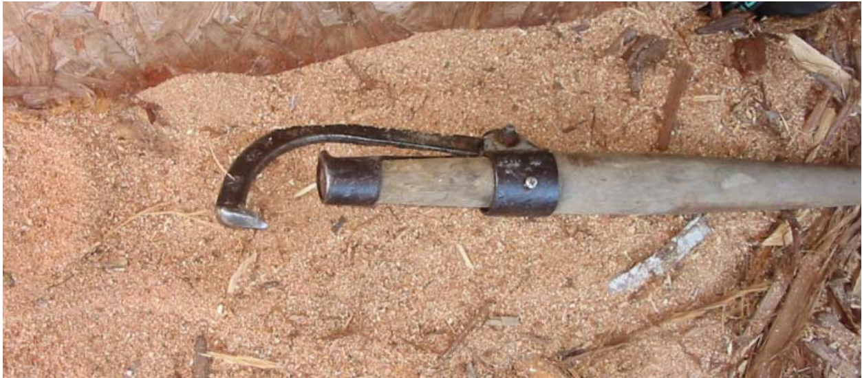
This peavey located at Monty Pfaff's mill was used to move logs by grappling and rolling them sideways.
