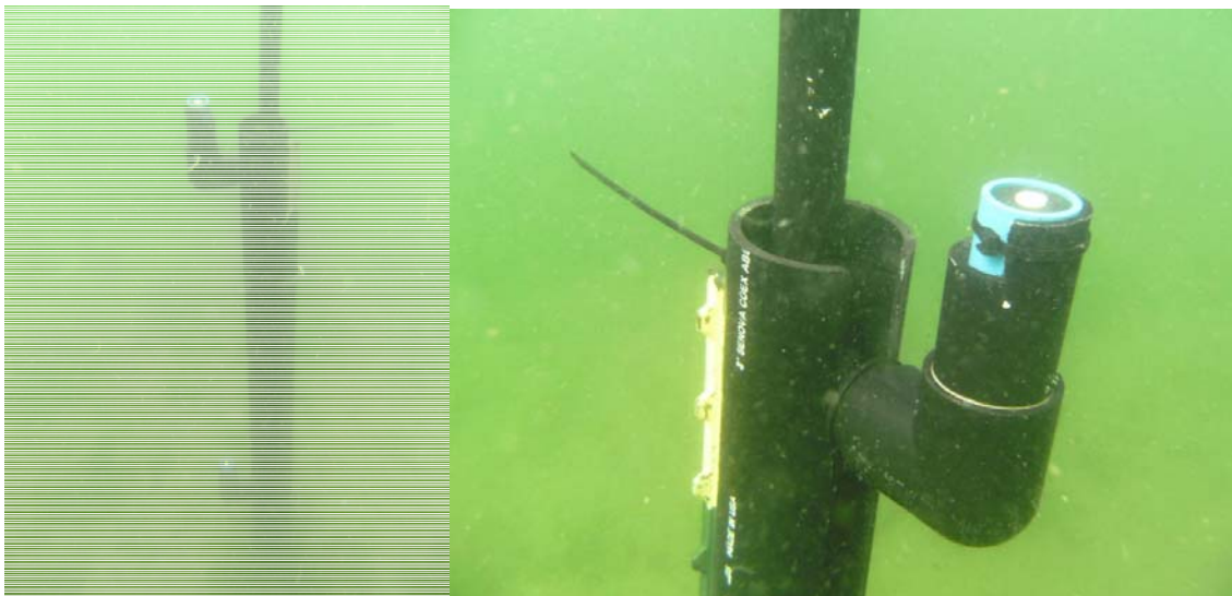
Figure 13. Odyssey light sensors deployed regionally near the eelgrass test plantings.
