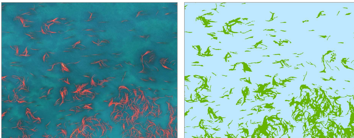
Figure 6. A small subsection of the P4 Multispectral orthomosaic (left; displayed as red edge, blue, green) at North Beach from the August 20, 2021 survey, and the results generated by the random forest classifier (right) of the same region. In the classified result, kelp canopy is symbolized as dark green and water/other as light blue.
