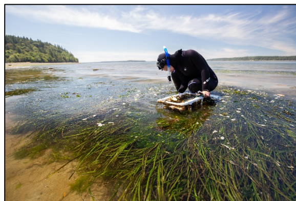
Figure 6. Water quality sensor array at Joemma Beach State Park being cleaned. Excessive fouling with epiphytes, barnacles, and macroalgae required cleaning. Sensors were cleaned on June 15 – 16, 2018 and on July 13, 2018.
