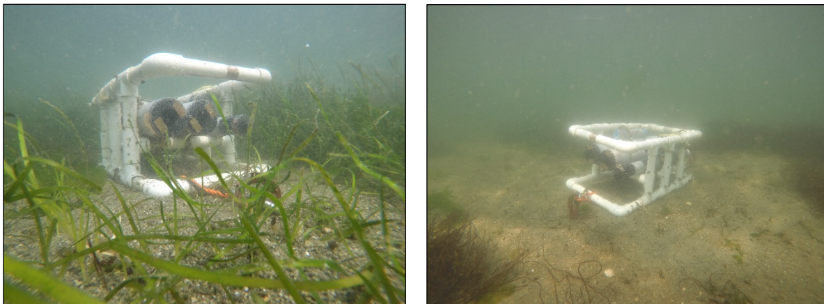
Figure 2. Water quality sensor array in large-scale eelgrass transplants (left) and adjacent unvegetated areas at Joemma Beach State Park.
