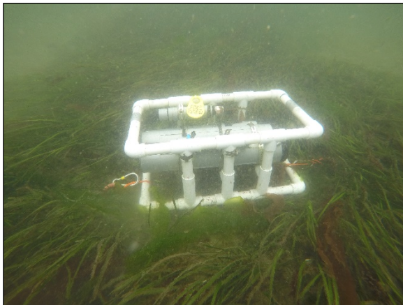
Figure 5. Example of sensor array deployed in transplanted eelgrass (left) and adjacent unvegetated, sandy areas (right) at Joemma Beach State Park in March 2018.
