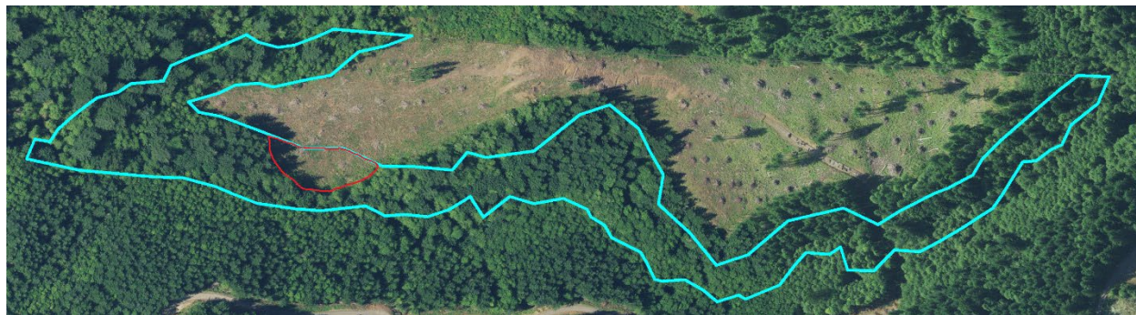
Figure 3.1a: Example of a forest management area (FMA) polygon with inaccurate spatial delineation. The boundary of the 14.8-acre FMA polygon is outlined in blue. The boundary of the 1-acre hardwood conversion within this FMA is outlined in red.
