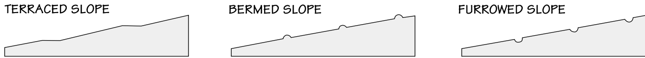
Figure 2.3. Small, discontinuous terraces, berms, and furrows can effectively slow runoff and decrease sediment transport. The relief is exaggerated for illustrative purposes. (From Banks, 1981.)
