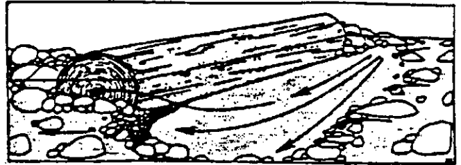
Figure 10. Lateral scour pool associated with large debris.
