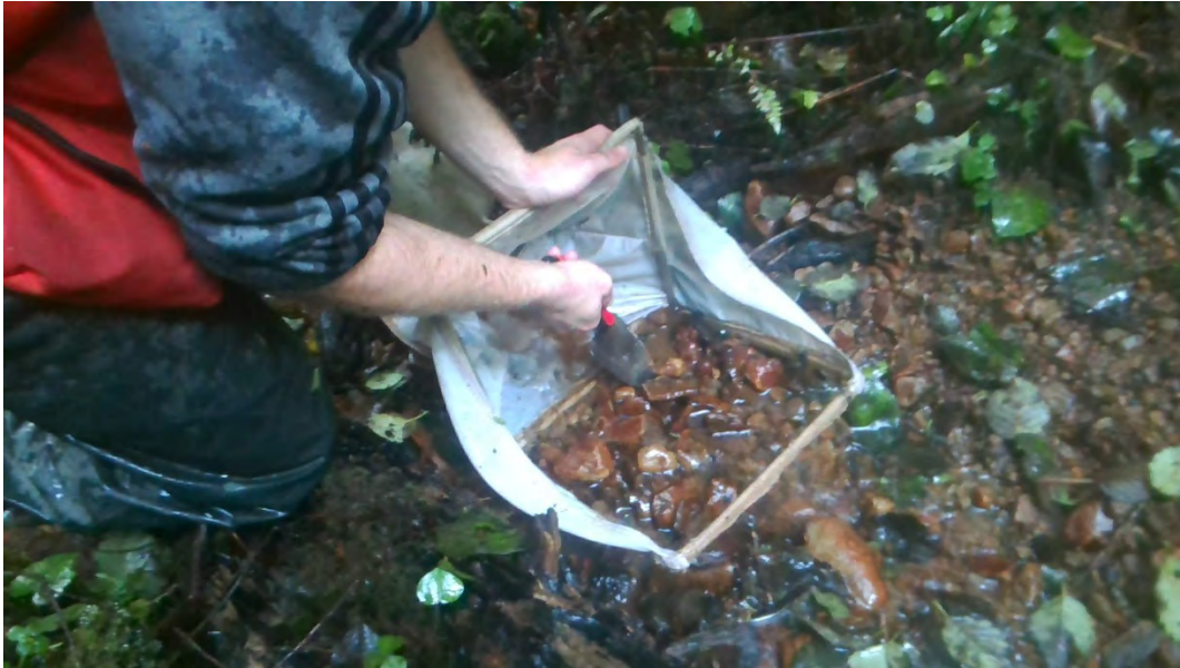
Figure 7-1. Surber sampler placement for sampling benthic macroinvertebrates. We collected the sample from the area designated by the sampler frame.
