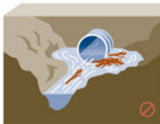
Figure 17 Design to prevent culvert plugging hazard
