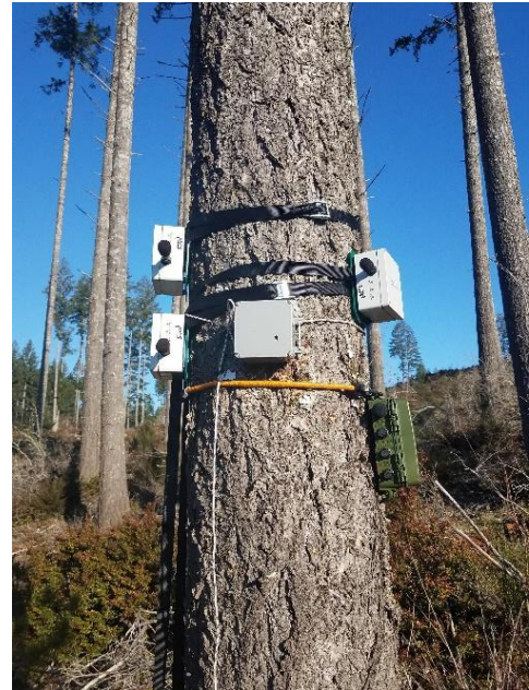
Figure 9: Detection Ranges of Different Models of Acoustic Recording Units are Compared as Part of the Passive Acoustic Monitoring Study. Photo courtesy of Teodora Minkova.
