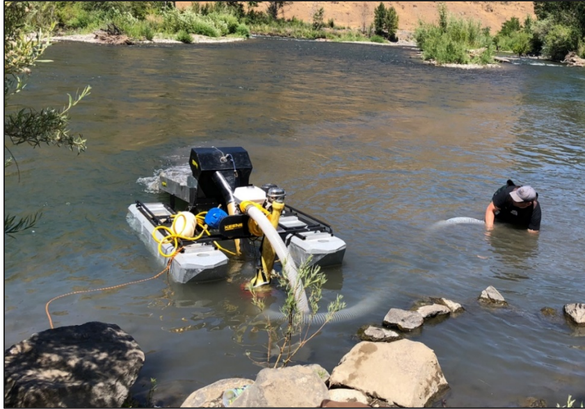
Figure 20. Trial run of the 5" suction dredge within the Little Naches River, Washington. Photo credit: Jaime Liljegen.
