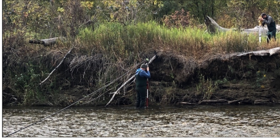
Figure 25. Elevation profiles were collected at five survey transects before, after, two months following the dredging experiment, and at the start of the next season in July 2019. These were visually assessed for direct vertical changes to the channel bed. Photo credit: Jaime Liljegren.
