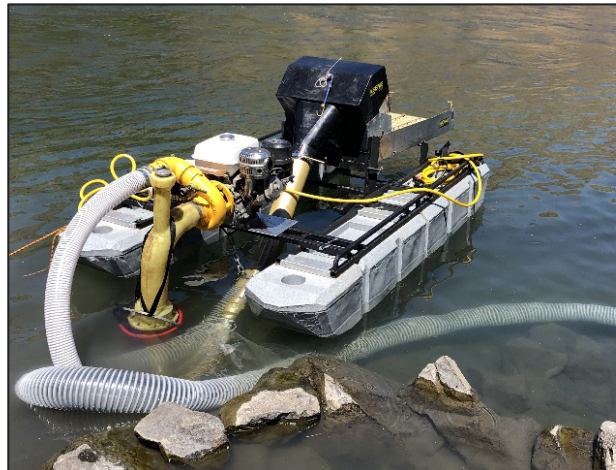
Figure 2. 5-inch Keene suction dredge with a pontoon framework, gasoline motor, water intake pump, and a header box to transport substrate over the attached sluice box for sorting. Photo credit: Jaime Liljegren.
