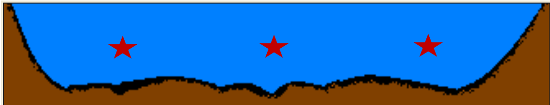
Figure 23. Channel cross-sectional diagram of approximate water quality measurement and turbidity sampling locations per identified transect. Vertically, samples were collected at 60% water depth of the water column. Horizontally, samples were collected at the 25%, 50% and 75% channel width distances. A total of three locations were measured and sampled per transect.
