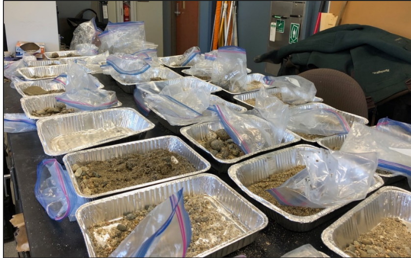
Figure 27. A subset of surficial bulk sediment samples collected during the study. Samples were dried at room temperature and then sorted to attain a present grain size distribution. Photo credit: Jaime Liljegren.
