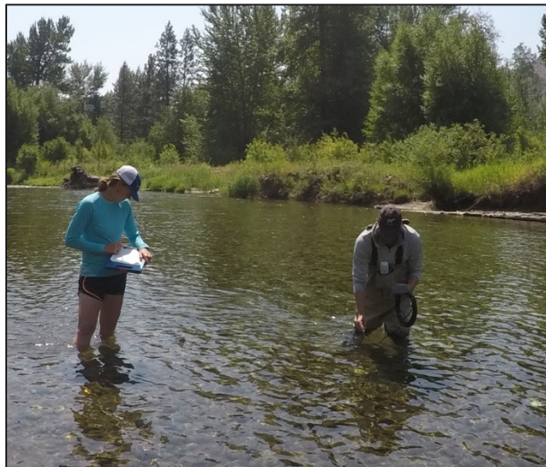
Figure 24. Survey assistants were deployed downstream at designated transects to monitor water quality parameters during dredging using a YSI 85 meter. Photo credit: Scott Kugel.
