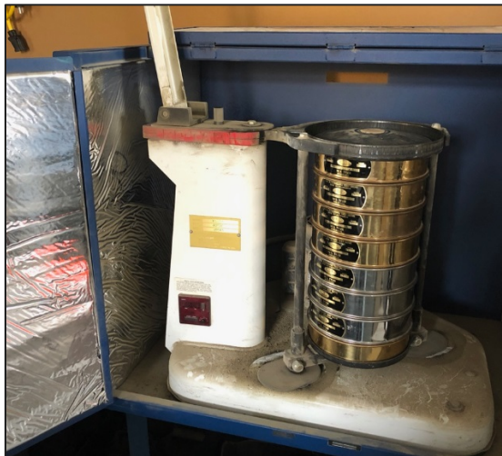
Figure 28. All bulk samples were processed through various sized sieves using a Ro-Tap sieve shaker in the Central Washington University Hydrology Lab. Photo credit: Jaime Liljegren.
