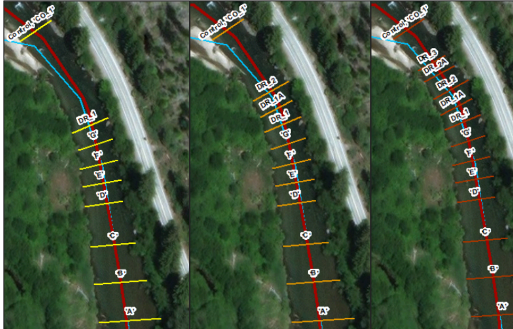
Figure 19. Monitored profiles over the three survey days. Dredge 1 was the general starting location for Day 1 along with Dredge 2 for Day 2, and Dredge 3 was for Day 3.
