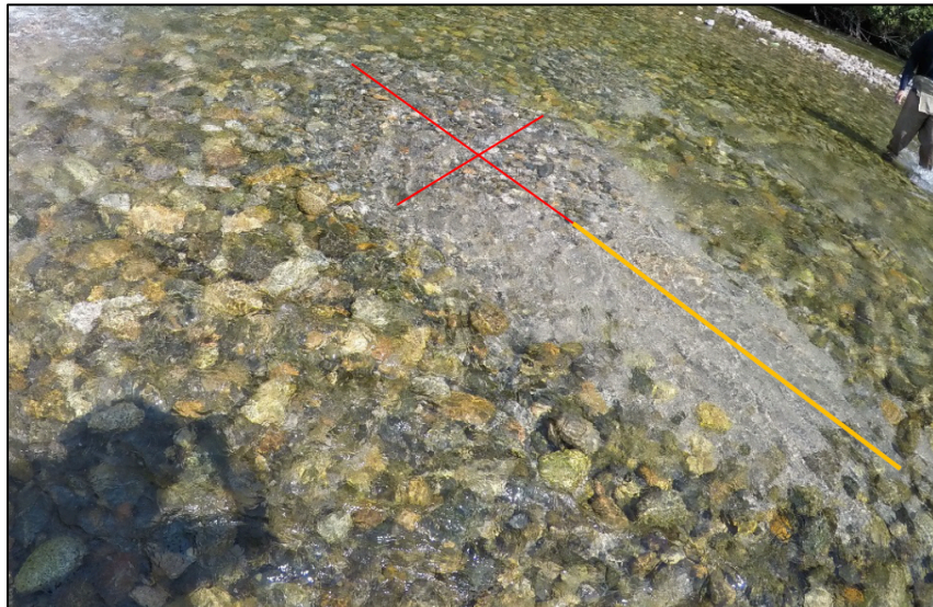
Figure 26. Length and width measurements of tailings pile created following dredging activity on Day 1 in the Entiat River, Washington. Grain sizes are sorted by water flow according to weight, with finer material transported further downstream. Photo credit: Scott Kugel.
