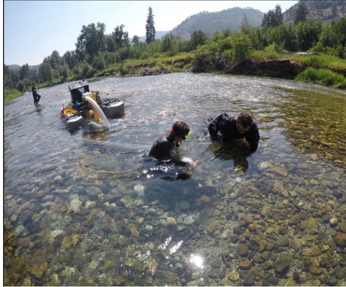
Figure 21. While the engine was in operation, two people were working the dredge with one person operating the suction hose while the other would move large material out of the dredge hole by hand and assist in the proper functioning and management of the dredge. Photo credit: Scott Kugel.
