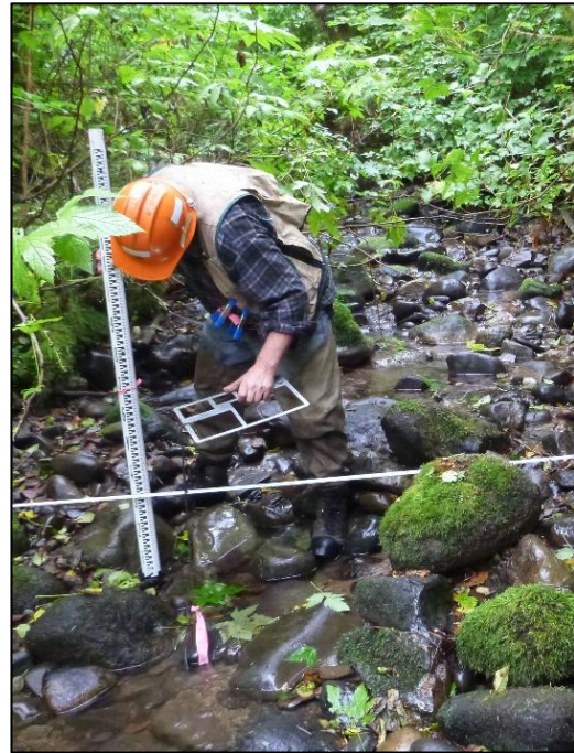
Using a gravelometer to measure the size of substrate particles
