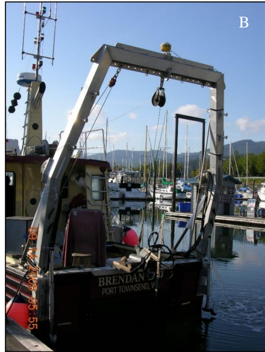
Figure 3: The R/V Brendan D II is equipped with a weighted towfish that contains an underwater video camera mounted in a downward looking orientation, dual lasers for scaling reference, and underwater lights for night work (A). The towfish is deployed directly beneath the DGPS antenna attached to the A-frame cargo boom, ensuring accurate geographic location of the camera (B).
