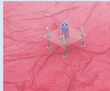
Submerged, mounted PAR sensor at bottom of water tank
