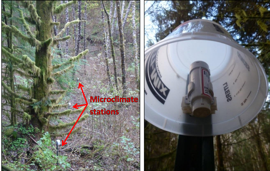
Figure 10-4. Part of a microclimate transect (left) and microclimate data logger and housing (right).
