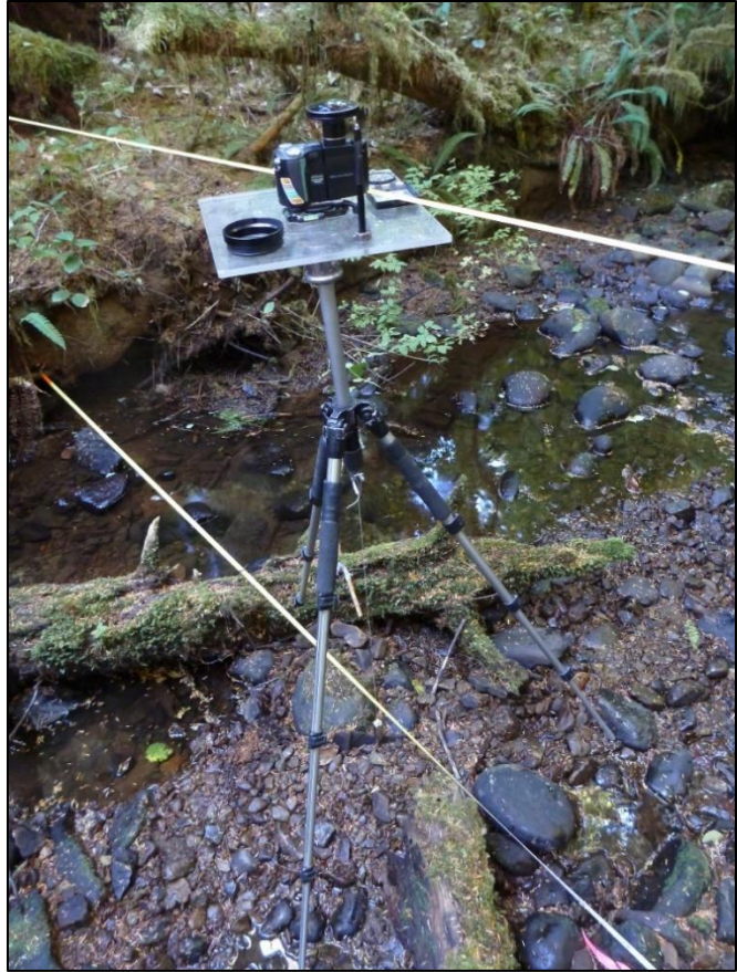
Figure 3-2. Camera positioned for a stream shade photo at the bankfull midpoint of a reach cross section.
