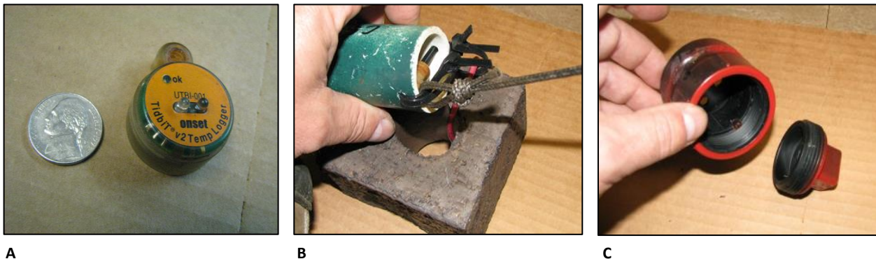
Figure 7-2. Assemble a temperature logger (A) in a PVC cover using nylon cable ties (for cord tether installations) (B) or a PVC cover (for epoxy mount installations) (C).
