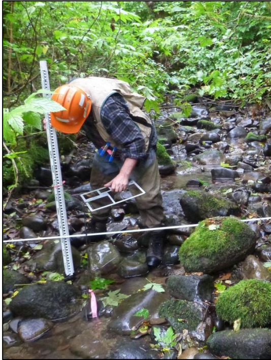
Figure 4-4. Sampling channel substrate using the stadia rod and gravelometer.
