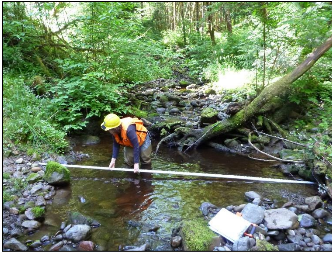
Figure 6-4. Measuring habitat unit wetted width (a) and maximum pool depth (b).
