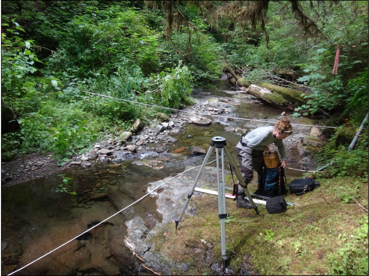
Figure 9-15. Channel hydraulics survey during summer low flow. The low flow control at is located about 5 meters downstream of the cross section. The reach extends roughly 10 meters up and downstream of the cross section. The channel is bedrock and rarely aggrades so the channel geometry and gauge survey are generally repeated only once a year. Other, less stable channels require surveys following most large flow events.
