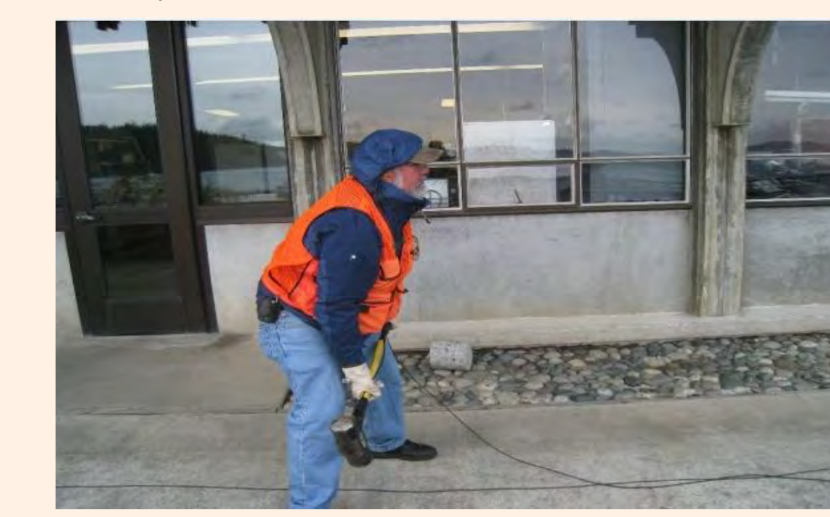
T. Walsh generates seismic energy using the sledgehammer at UWFH.
