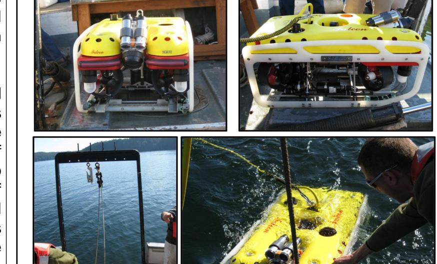
Remotely operated vehicle (ROV) – paired lasers mounted on top of camera (front and side views on top figures), lowering and early testing the elements of the ROV (bottom pictures)
