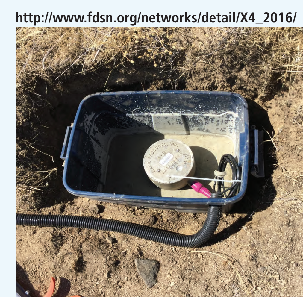
L-22 3-component short-period Sensor (2 Hz, 0.70 damping, 88 W/m/s sensitivity)
