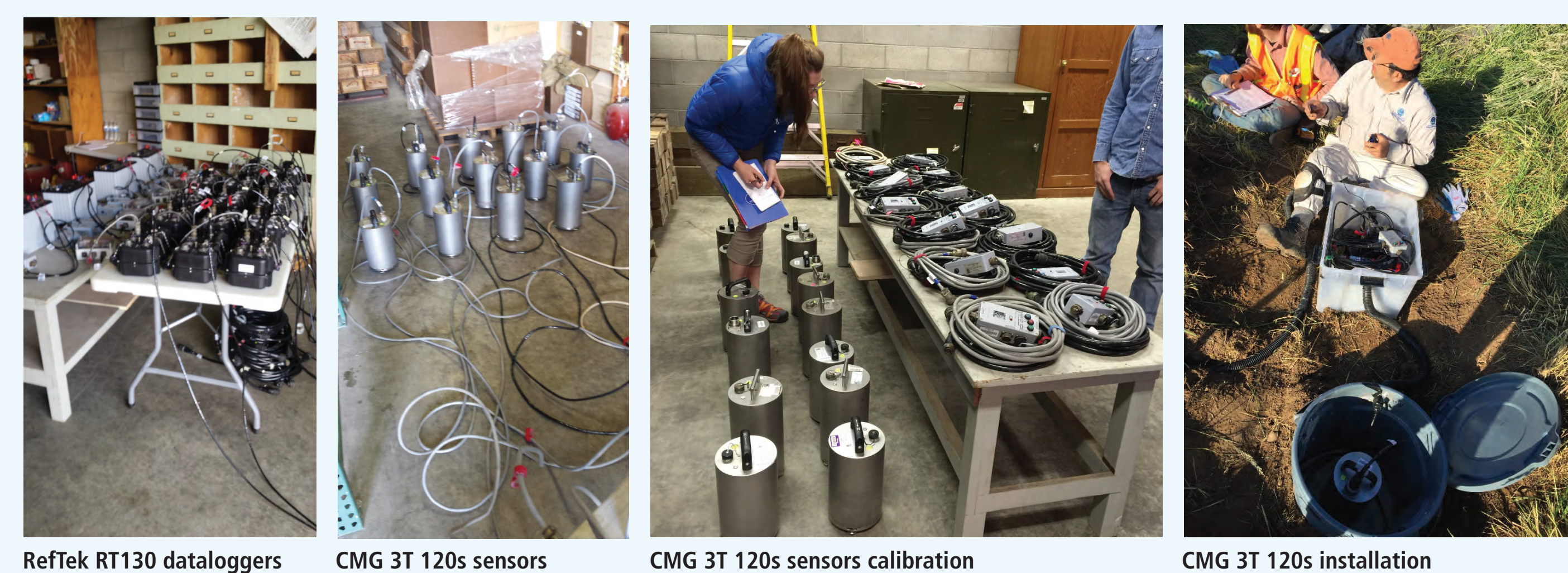
Reftek RT130 dataloggers CMG 3T 120s sensors CMG 3T 120s sensors calibration CMG 3T 120s installation Guralp CMG-3T Broadband (120s -50Hz flat velocity response, with remote electronic mass locking, unlocking, and centering)
