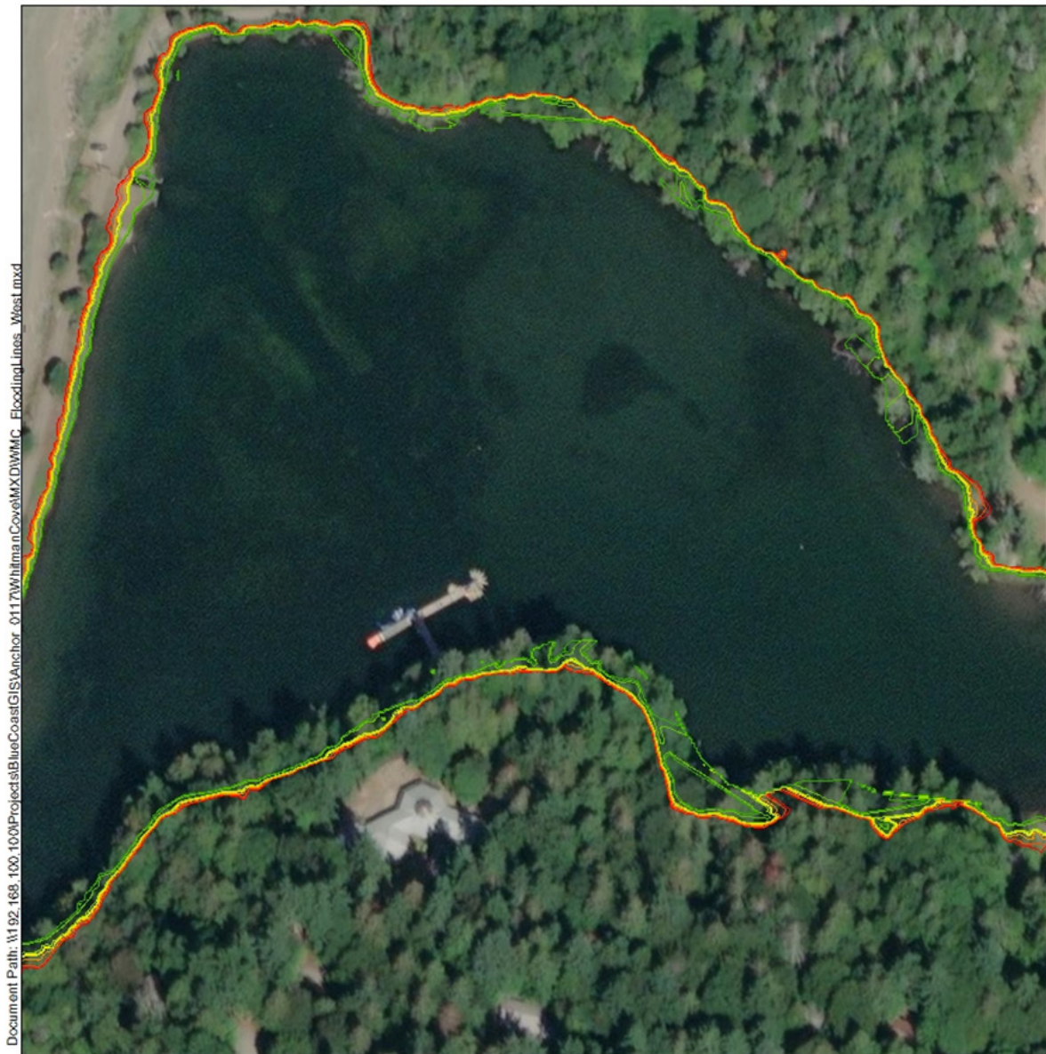
Figure 18 Flooding Potential, West End of Cove
