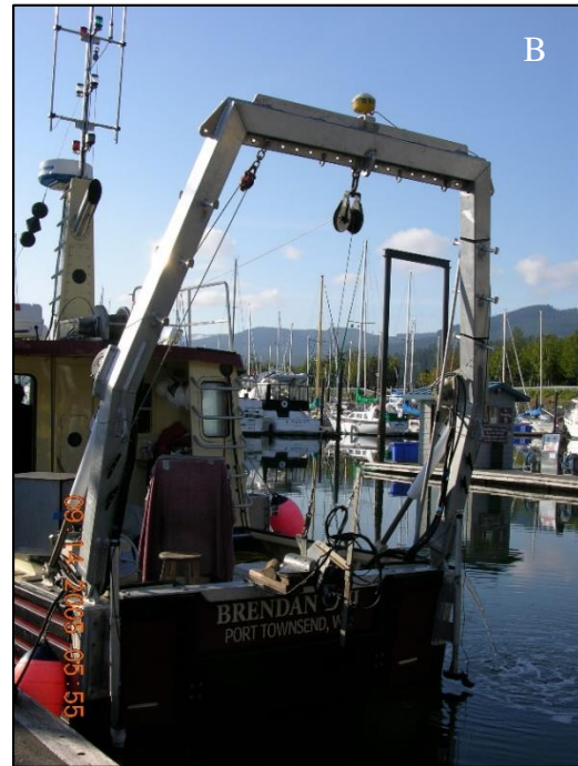
Figure 2: The R/V Brendan D II is equipped with a weighted towfish that contains an underwater video camera mounted in a downward looking orientation, dual lasers for scaling reference, and underwater lights for night work (A). The towfish is deployed directly beneath the DGPS antenna attached to the A-frame cargo boom, ensuring accurate geographic location of the camera (B).
