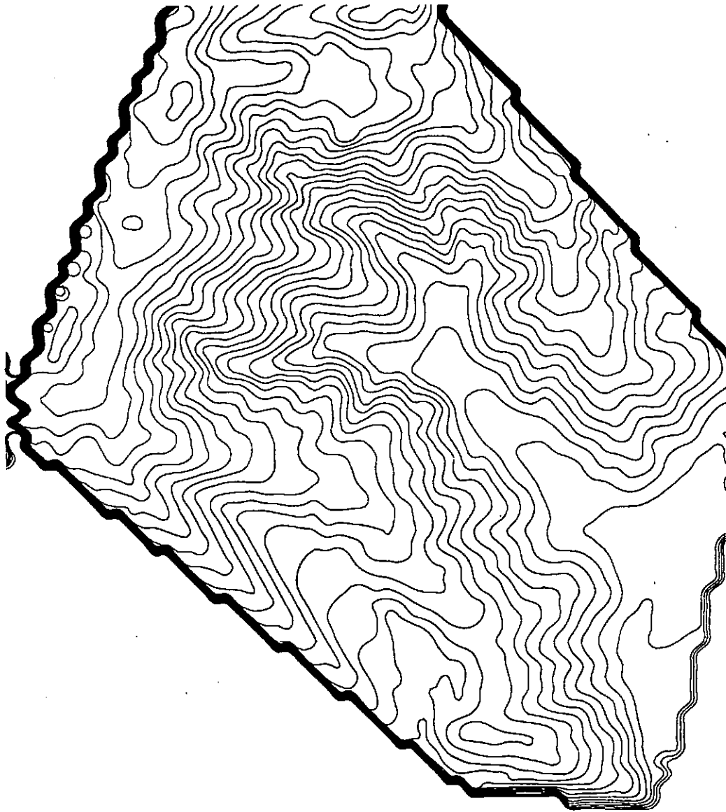
Figure 1: Tennessee Valley from hand-digitized points, 30m grid spacing contour interval 10 m, 1" = 330m
