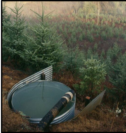
Figure 7. A photograph of a sediment tub installed below a road segment.
