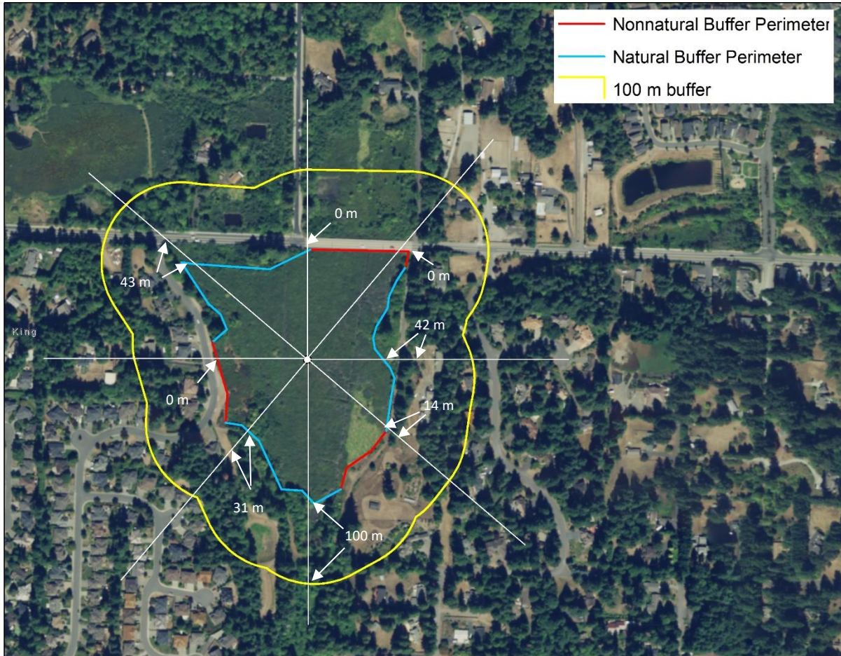
Figure 6. Buffer Width Calculation (point-based or simply polygons). The length of natural buffer is measured by calculating the distance between the edge of the AA and the 100 m buffer line along each of the eight white lines. Then an average is taken. In this example the calculation for average buffer length is (moving clockwise): (0+0+42+14+100+31+0+43)/8=28.75 m (Table 16). Consulting Table 18 this translates to a “C” rating.
