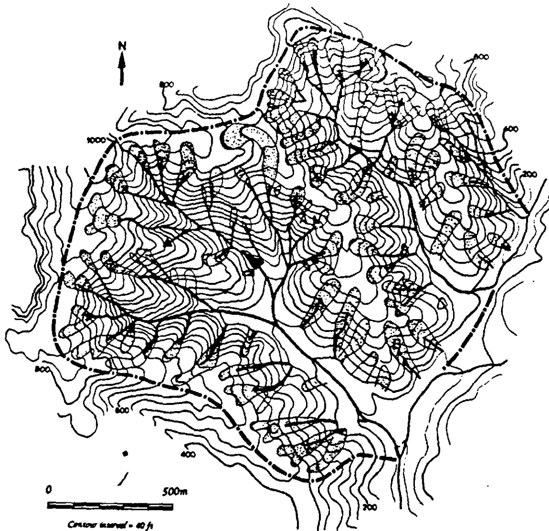
Figure 2: Channels and colluvial deposits in the Tennessee Valley of Marin County, California. Both continuous and discontinuous channels are indicated by heavy black lines and the approximate extent of colluvial deposits are indicated by the stippled areas. Small triangle in middle left of the figure represents a channel head associated with a road drainage culvert. The black pattern in the area near center of figure denotes a man-made pond (from Montgomery and Dietrich, 1989).
