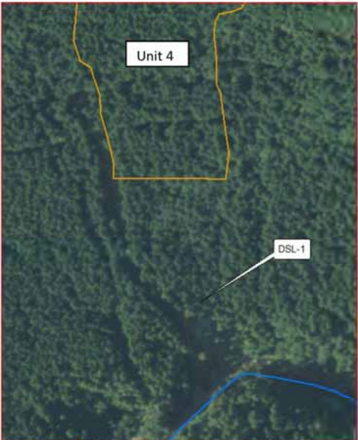
Image 6: 2009 orthophotograph showing appearance of debris flow track from CD-0201 road.
