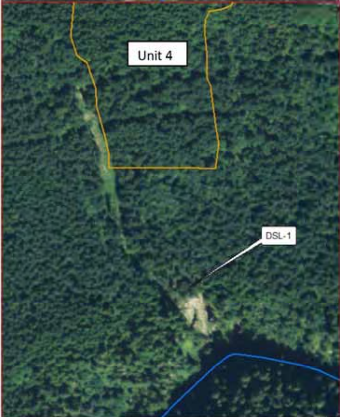
Image 7: 2011 orthophotograph showing debris flow track from CD-0201 road.
