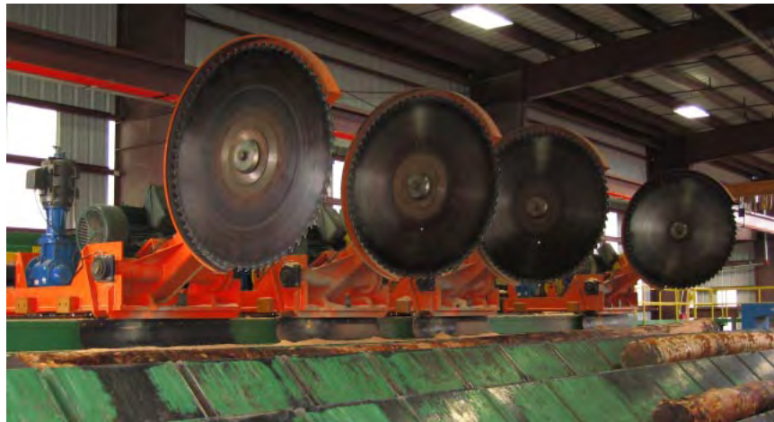
A "merchandise" is equipped with several saw blades to quickly cut lumber to a variety of custom lengths. Photo: Sierra Pacific Industries / Sheri Nelson
