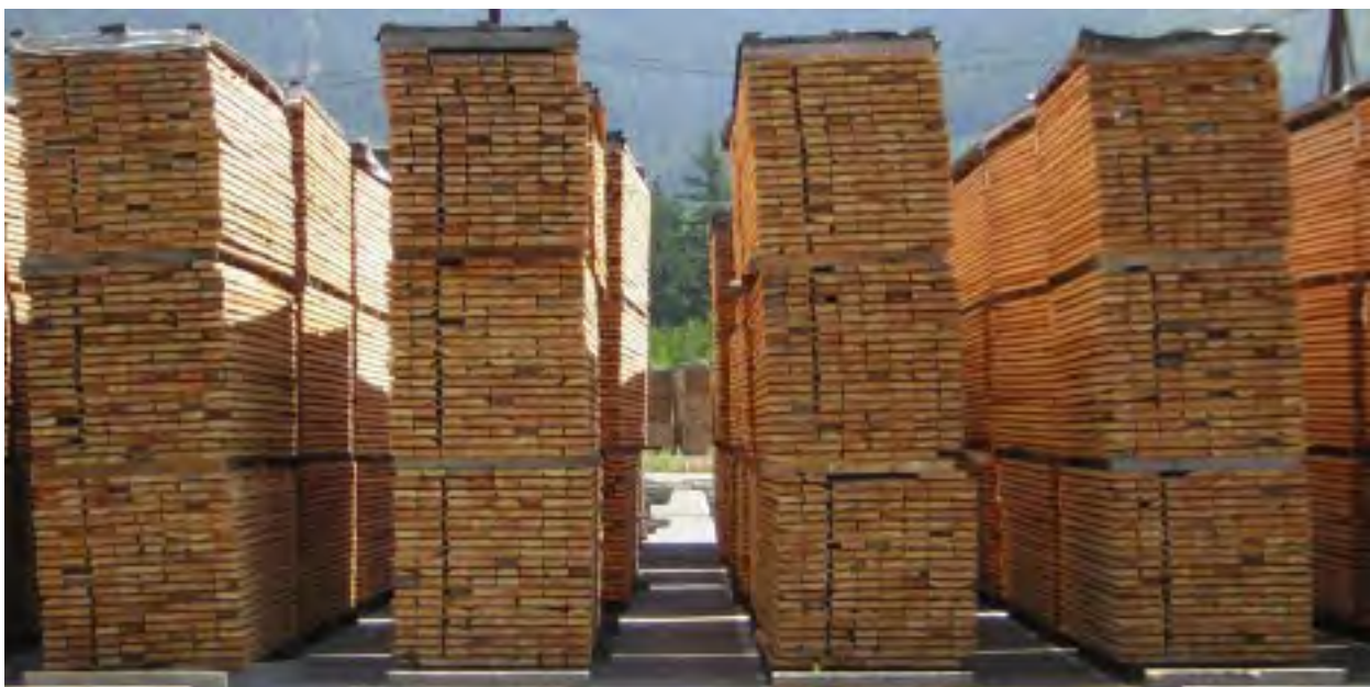
Douglas fir dimensional lumber (2" x 6") stacked at Great Western Lumber Company in Whatcom County. Photo: DNR/ Dorian Smith
