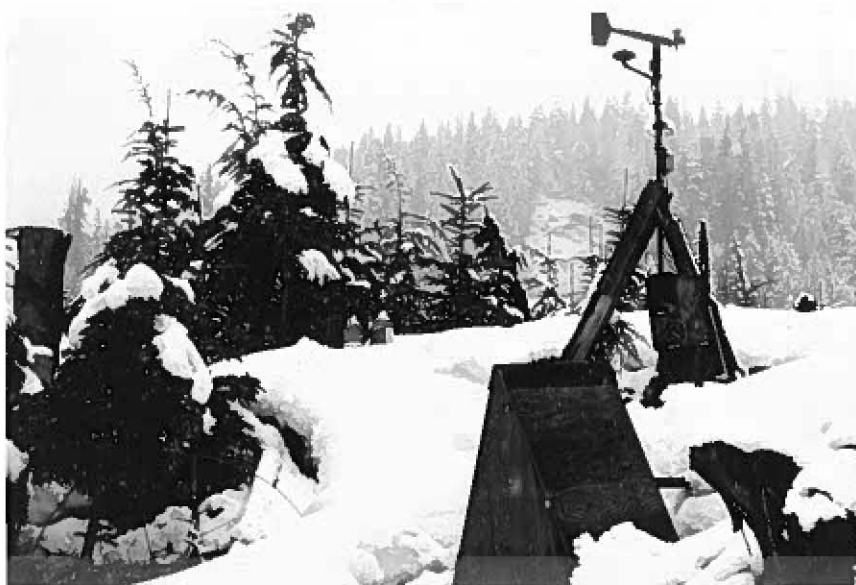
Figure 9. Weather station at the 760-m (2500-ft) clearcut plot at Finney Creek, March 22, 1989. The rain gauge is located at the far left, and the snow collector is located out of the photograph to the right.
