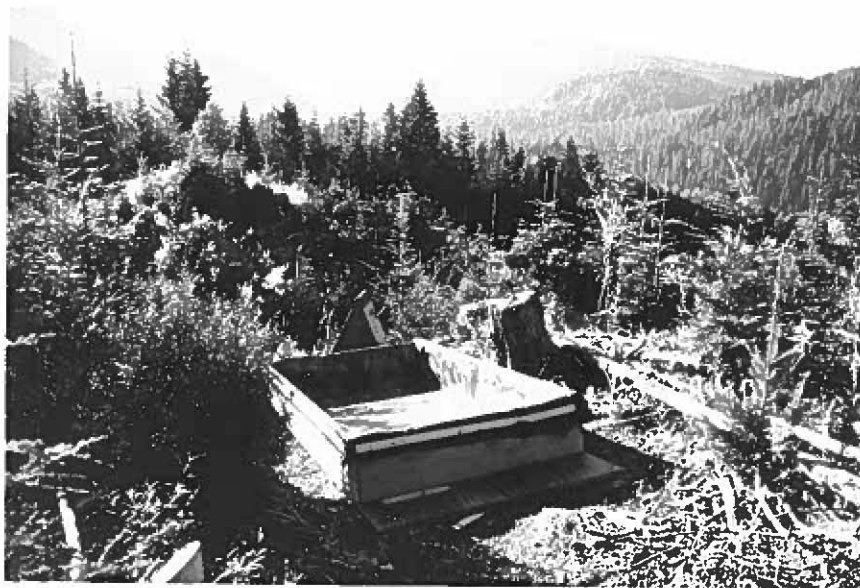
Figure 4. Snow is collected in boxes located on nearly level ground to prevent damage to boxes from snow creep and to minimize measurement errors caused by flow of melt water being altered by sloping ice lenses in the snowpack.
