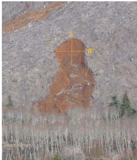
Figure 7. Photograph from Post-Mortem Field Manual that illustrates how to measure the failure initiation dimensions. (Photograph: Julie Dieu)
