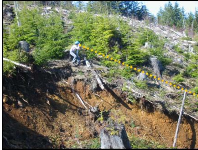
Figure 2. Example of measuring hillslope gradient at the failure initiation site (from Post-Mortem Field Manual Photo: Julie Dieu).
