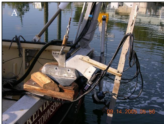
Figure 4: The R/V Brendan D II is equipped with a weighted towfish that contains an underwater video camera mounted in a downward looking orientation, dual lasers for scaling reference, and underwater lights for night work (A). The towfish is deployed directly beneath the DGPS antenna attached to the A-frame cargo boom, ensuring accurate geographic location of the camera (B).
