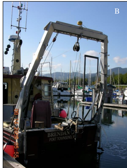
Figure 5: The R/V Brendan D II is equipped with a weighted towfish that contains an underwater video camera mounted in a downward looking orientation, dual lasers for scaling reference, and underwater lights for night work (A). The towfish is deployed directly beneath the DGPS antenna attached to the A-frame cargo boom, ensuring accurate geographic location of the camera (B).
