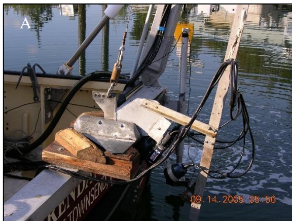
Figure 5: The R/V Brendan D II is equipped with a weighted towfish that contains an underwater video camera mounted in a downward looking orientation, dual lasers for scaling reference, and underwater lights for night work (A). The towfish is deployed directly beneath the DGPS antenna attached to the A-frame cargo boom, ensuring accurate geographic location of the camera (B).
