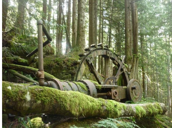
Pelton wheel, used to power historic mines in DNR's Northwest region. Photo: DNR
