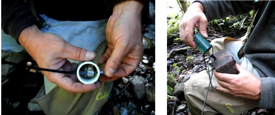
Figure 4. Left: water temperature data logger setup zip tied into a protective PVC housing. Right: complete setup with data logger, anchor brick, zip ties, PVC housing, and nylon cord.
