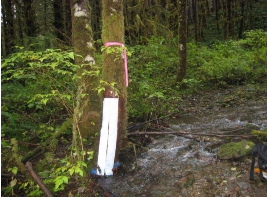
Figure 8. An example of a Velcro strips installation (basin 619).
