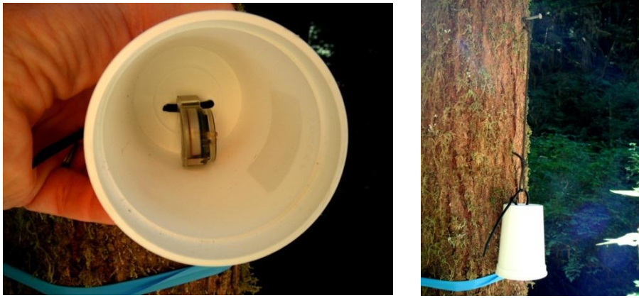
Figure 5. Left: Air temperature data logger setup, view from inside the cup. Right: Complete air temperature data logger setup, mounted on north side of a tree.
