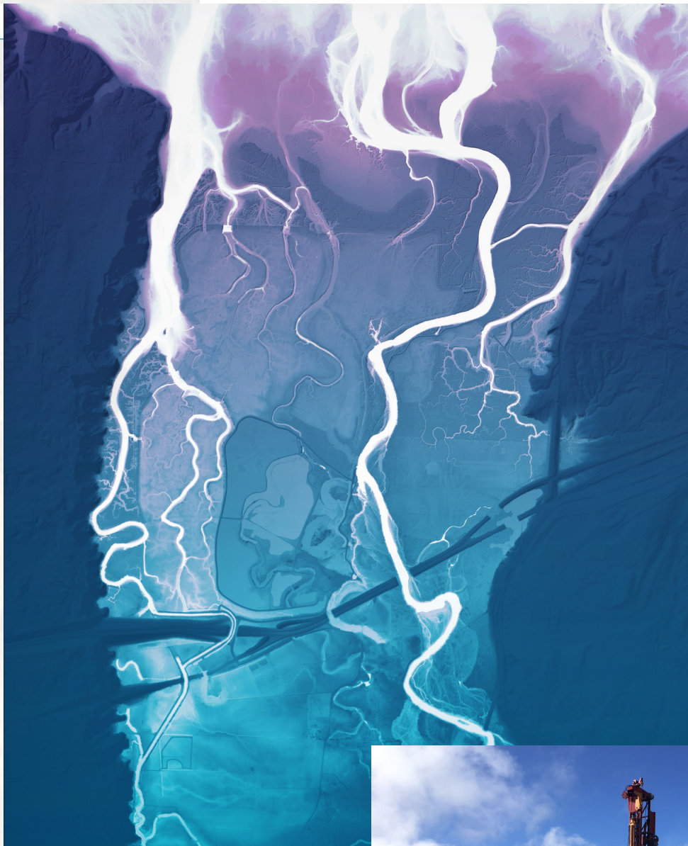
Figure 10. Lidar topography and bathymetry of the Nisqually Delta. Lidar reveals complex estuarine topography relevant to salmon and environmental factors.
