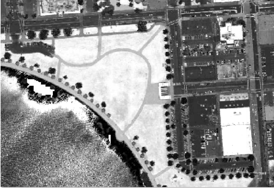
Figure 17. Intensity image. Intensity images represent the strength of the returned measurement to the lidar system.
