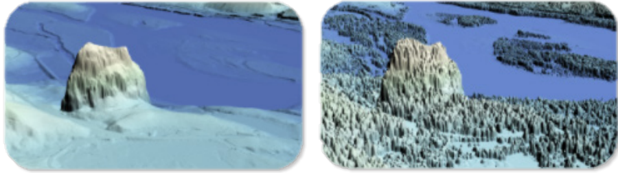
Figure 16. Example of a bare earth DEM (left), vegetation and structures are removed. Example of a first-return DEM (right), which includes vegetation and man-made structures.
