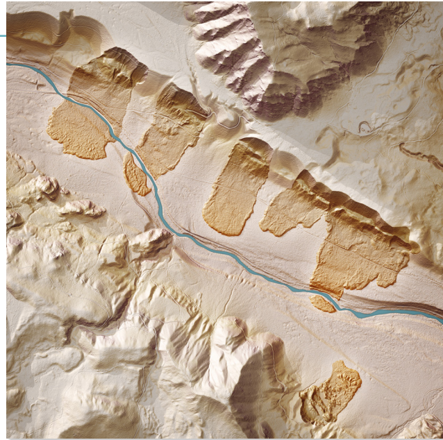
Figure 6. Comparison of imagery and lidar data over Cedar River, King County. Lidar data reveal several landslide features beneath the vegetation.
