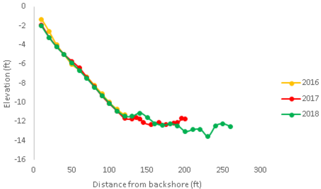
Figure 17. Beach elevation profile for Custom Plywood, FBAR from 2016-2018 surveys.
