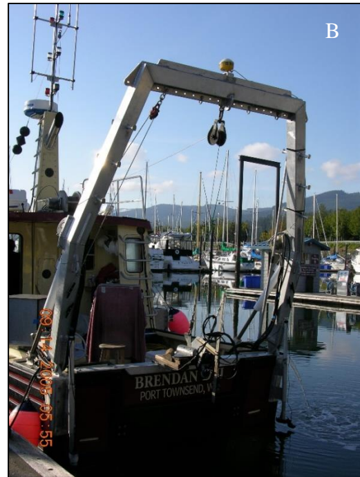
Figure 4: The R/V Brendan D II is equipped with a weighted towfish that contains an underwater video camera mounted in a downward looking orientation, dual lasers for scaling reference, and underwater lights for night work (A). The towfish is deployed directly beneath the DGPS antenna attached to the A-frame cargo boom, ensuring accurate geographic location of the camera (B).
