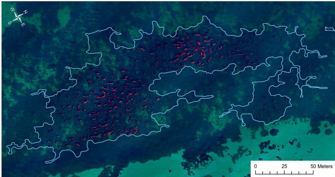
Figure 1. Example of two floating kelp metrics, illustrated in aerial imagery. The floating kelp bed area metric tracks the perimeter of the forest floating on the surface (the blue polygon), which includes kelp individuals and gaps between them. Another common metric is canopy area (the red features within the polygon in the near infrared imagery), which includes floating individuals but excludes gaps between individuals. In Washington State, bed area data is more spatially and temporally extensive. At many locations, the floating kelp monitoring program tracks canopy area in addition to bed area. All available parameters are considered during trend assessment.
