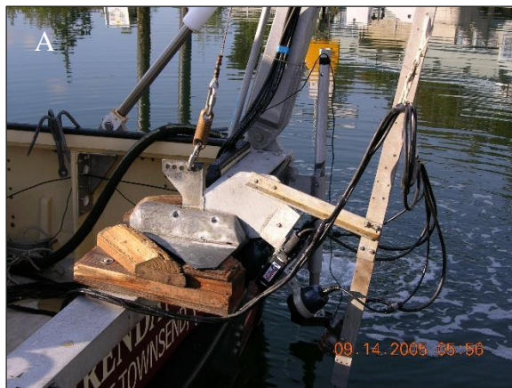
Figure 3: The R/V Brendan D II is equipped with a weighted towfish that contains an underwater video camera mounted in a downward looking orientation, dual lasers for scaling reference, and underwater lights for night work (A). The towfish is deployed directly beneath the DGPS antenna attached to the A-frame cargo boom, ensuring accurate geographic location of the camera (B).
