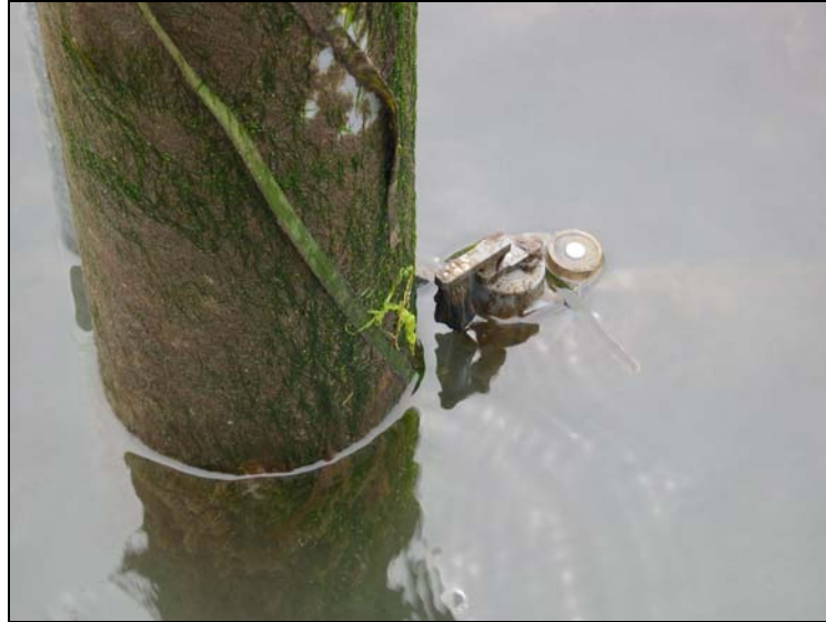
Figure A-12. Photo of upper PAR sensor at WP in air during a low tide at 10:25 PDT 6/15/07.
