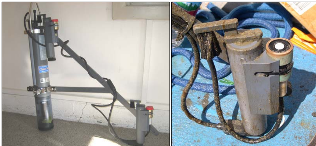
Figure 2-1. The YSI 6600 EDS with dual PAR kit (left) and a close-up of the lower PAR sensor and wiper with fouling accumulated over 3 weeks and 4 days in Westcott Bay.
