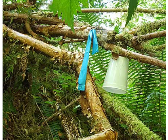
Photo 1. Air temperature sensor installed near a stream in the OESF.
