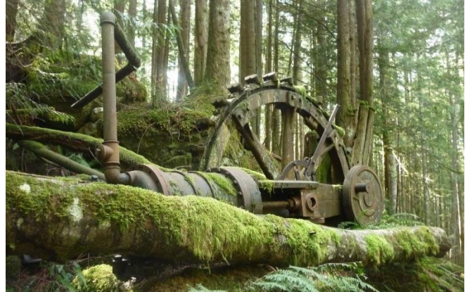
Pelton Wheel, Used to Power Historic Mines in DNR's Northwest Region. Photo: DNR
